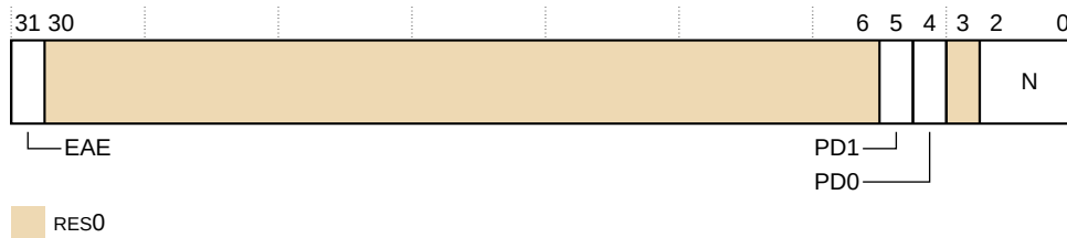
Figure 3-72: TTBCR bit assignments, TTBCR.EAE is 0
