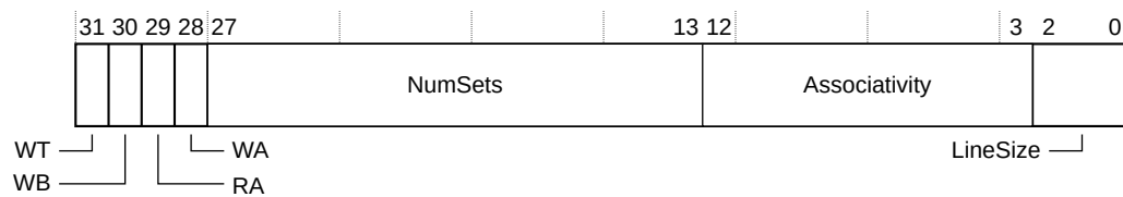
Figure 3-11: CCSIDR bit assignments
