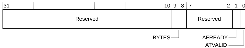
Figure 5-85: TRCITIATBOUTr bit assignments
